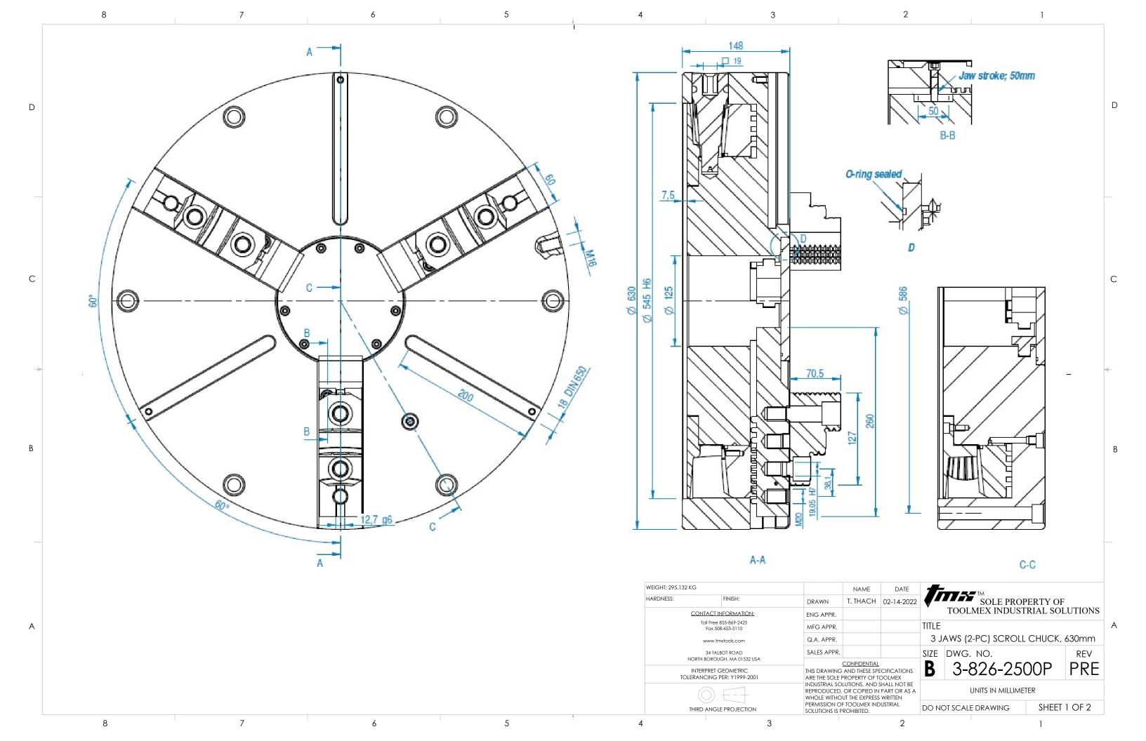
TECHNICAL SPECIFICATIONS Torque on key 40 Da.N.m D 10000 DaN Gripping force Steel F-II4 Material 970 r.p.m Max. Speed Rotation WEIGHT: 295.132 KG NAME DATE
