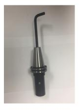
Insert allen wrench into taper and loosen draw bar screw.
